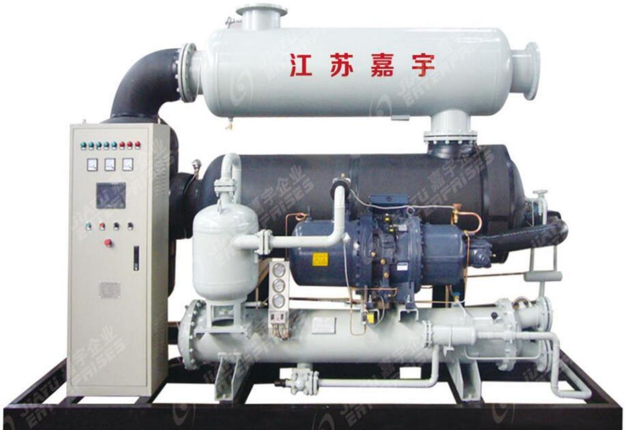
**JLD series refrigerating air dryer** is a kind of compression refrigeration technology that uses forced cooling of compressed air to make water vapor, oil mist and other condensed liquid droplets discharged from the machine by automatic drainer, thus obtaining a more pure compression air. JLD Series Refrigerating Air Dryer use international famous brands of compressors and key refrigeration components, reliable performance, stable operation, low noise, light and beautiful appearance.
